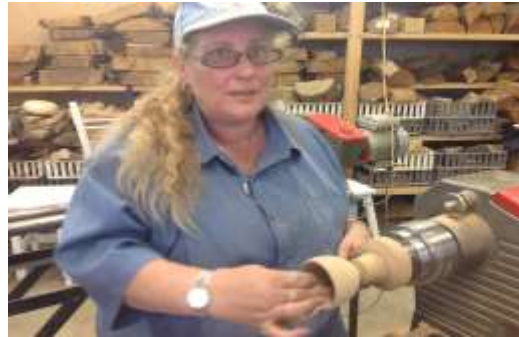
Alice has completed shaping the top part of a goblet. Now comes the sanding and finishing of the bowl bit. Next the base then the stem.
