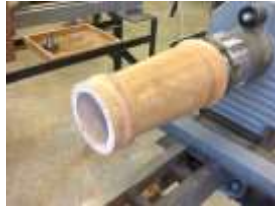
David slowly removed the core of his tall pot using a series of Forstner drill bits.
