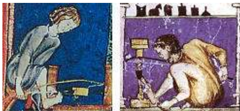
Fig 9: Turning on the bow lathe in 1283
