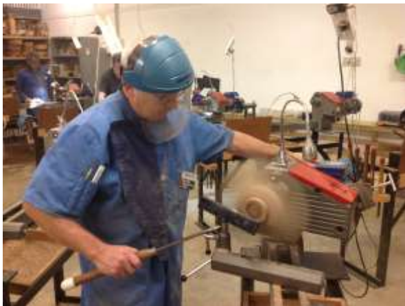
MURRAY is careful to take a wide berth when reaching around his rapidly spinning winged bowl.
