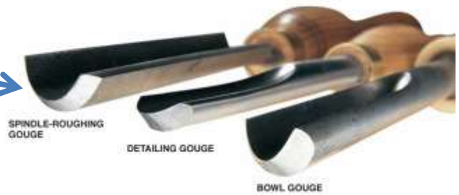
Roughing gouges set at 45 Degrees
